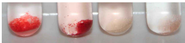
Figure 2. Treatment of Wang resin (Fluka, 1.1 \text{ mmol g}^{-1} ) with (from left to right): NF31/DMAP at rt; NF31/DMAP at 70^\circ\text{C} ; NF31 at rt; NF31 at 70^\circ\text{C} . 18,20
