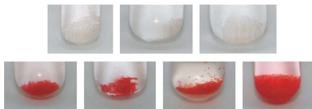
Figure 3. Resin appearance after treatment with NF31/DMAP: 20 top (from left to right): 2-chlorotritylchloride resin (Iris Biotech GmbH, 1.55 \text{ mmol g}^{-1} ), carboxy polystyrene (Novabiochem, 0.98 \text{ mmol g}^{-1} ), Merrifield resin (Novabiochem, 1.0 \text{ mmol g}^{-1} ); bottom (from left to right): aminomethylated polystyrene (Novabiochem, 1.1 \text{ mmol g}^{-1} ), HMPB-MBHA resin (Novabiochem, 0.51 \text{ mmol g}^{-1} ), Novasyn ® TG HMP resin (Novabiochem, 0.25 \text{ mmol g}^{-1} ), Kaiser oxime resin (Novabiochem, 1.3 \text{ mmol g}^{-1} ).
